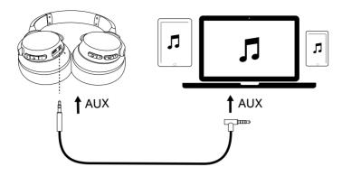
Plugging in an audio cable will automatically switch to AUX mode, and Bluetooth mode and ANC will turn off.
